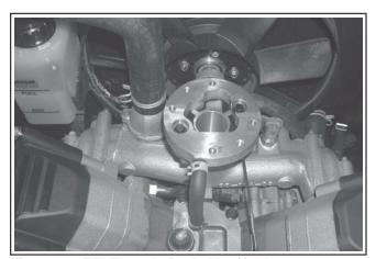
Figure 27. EFI Throttle Body Manifold.
